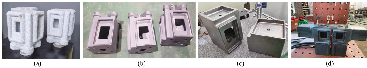
Fig. 7. Fabrication process of the modular nodes (a) 3D-sand printed mold; (b) metal casting mold (c) raw nodes; (d) S-CN connections.
