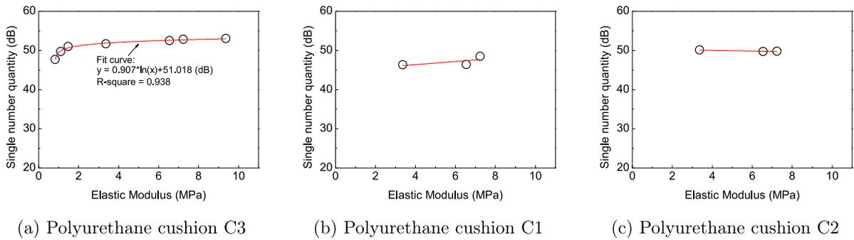
Fig. 11. The relationship between elastic modulus and impact sound performance of the full-filled novel floating floors.
