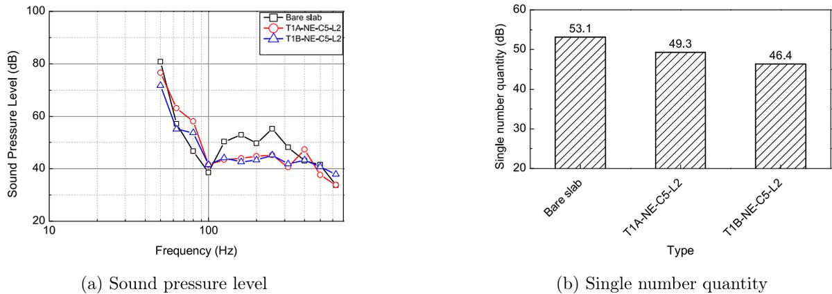
Fig. 18. Impact of the lightweight concrete layer on sound response in the full-filled floating floors.
