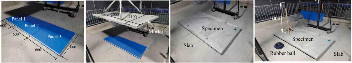
(a) Place three panels without the mortar layer centrally on the second floor.
