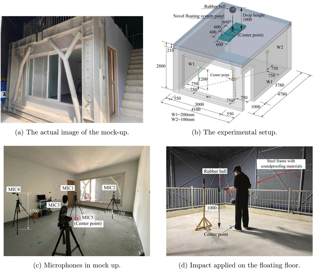
Fig. 5. The experimental setup for impact sound measurement.
