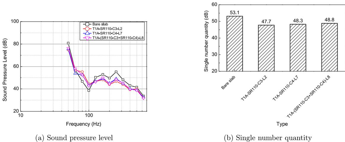
Fig. 12. Impact of polyurethane cushion arrangement on sound response of the full-filled novel floating floors.
