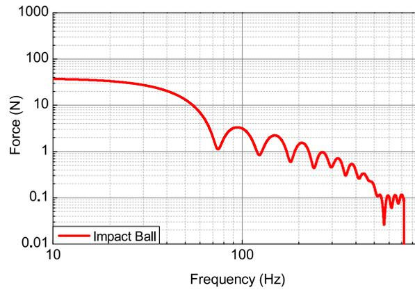
Fig. 6. Force spectrum of the impact ball.
