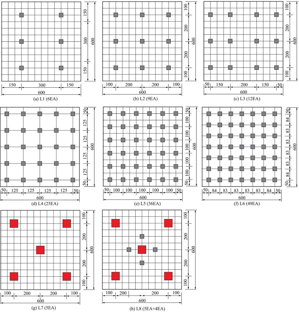
Fig. 4. Arrangement of polyurethane cushions in the panel.
