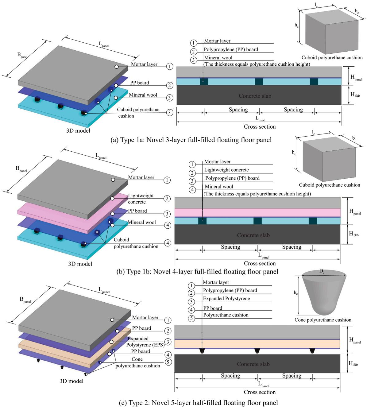
Fig. 2. Configuration and cross-section of a module of novel floating systems.
