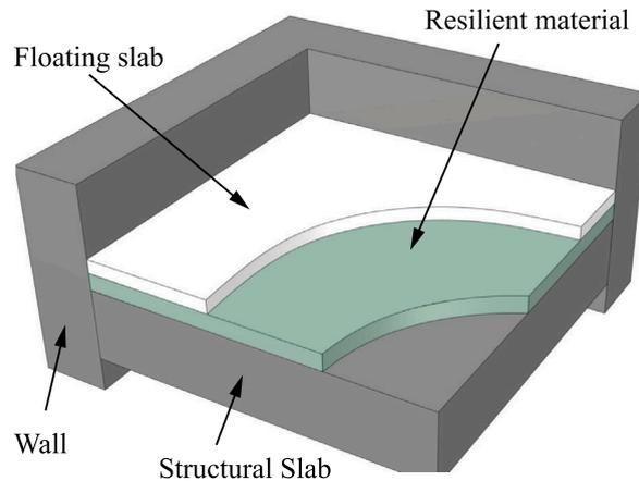
Fig. 1. Typical floating floor system.
