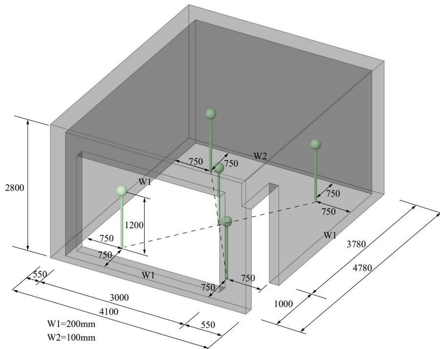
Figure 3: The schematic diagram of the experimental facility used for the impact sound measurement.
