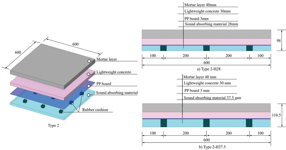
Figure 2: Configuration and cross-section of a module of the tested floating floor Type 2.
