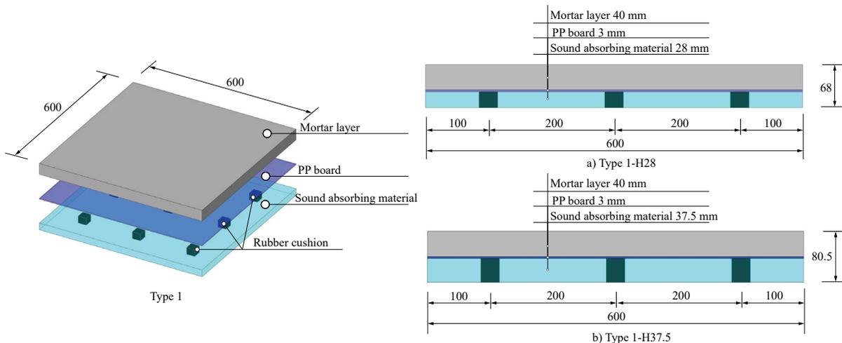
Figure 1: Configuration and cross-section of a module of the tested floating floor Type 1.
