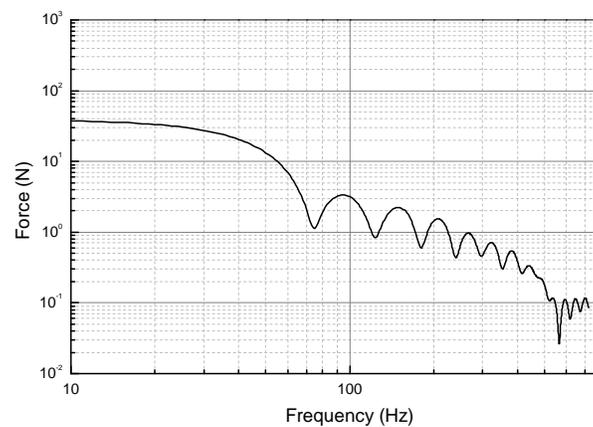
Figure 5: Force spectrum of the impact ball.
