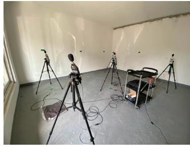
(b) The microphones installed in the receiving room under the load-bearing slab.
