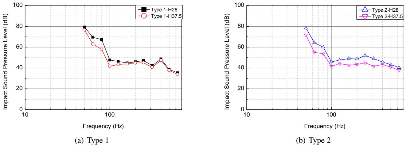
Figure 6: The influence of the height of the rubber cushions on the acoustic performance of the novel floating floor.
