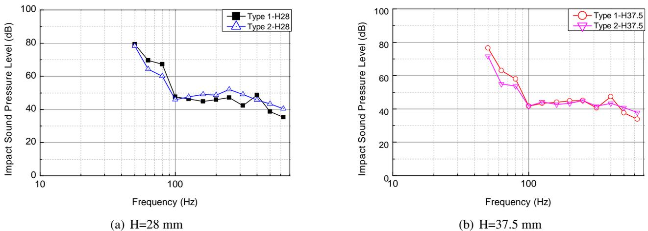
Figure 7: The influence of the lightweight concrete layer on the acoustic performance of the novel floating floor
