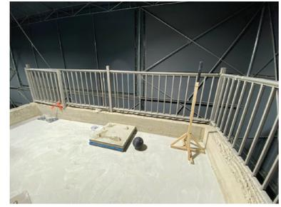
(c) The standard impact source (rubber impact ball) and an unit of a novel floating floor.
